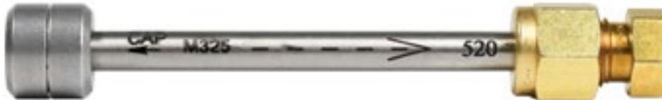
Tube with diffusion cap in place for sampling
