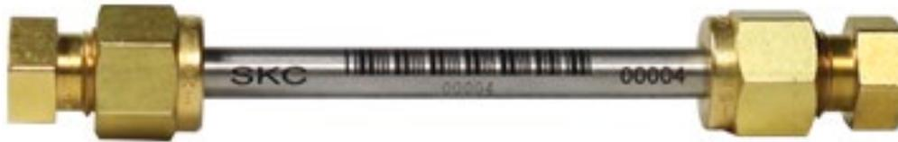
Tube sealed with Swagelok
